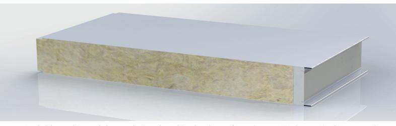
Sandwich panel in steel sheet and mineral wool insulated core, fire resistance 45 minutes. Used for external cladding, internal partitions, false ceilings and in general wherever good mechanical bearing capacity is required.
