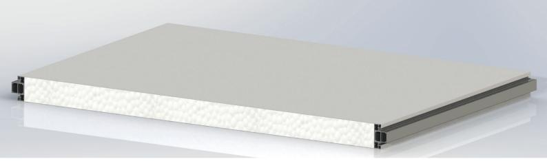
Sandwich panels insulated with glued expanded polystyrene and with aluminum perimeter frame, used to create average/high level clean rooms thanks to the easy cleaning of the walls, the excellent aesthetic finishing and its low cost.
